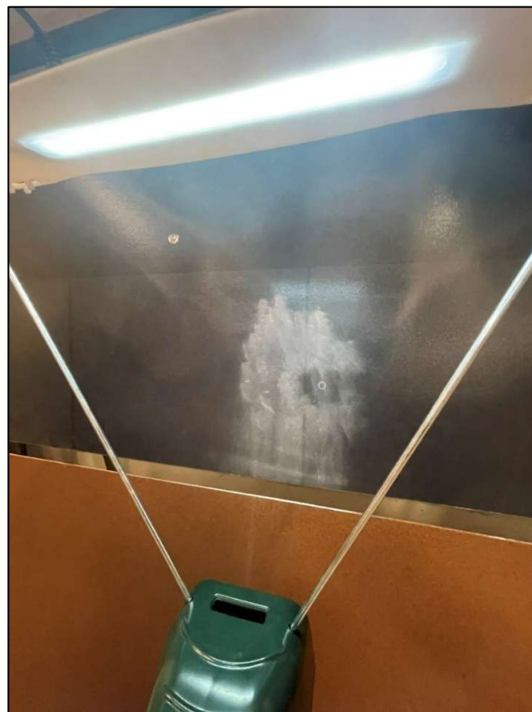
Figure 10 – Talcum used to better specify the impact location.
