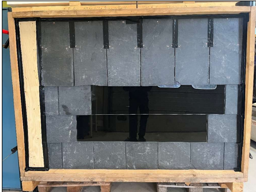
Figure 1 – Front of the test specimen mounted in the wind pressure test rig.
