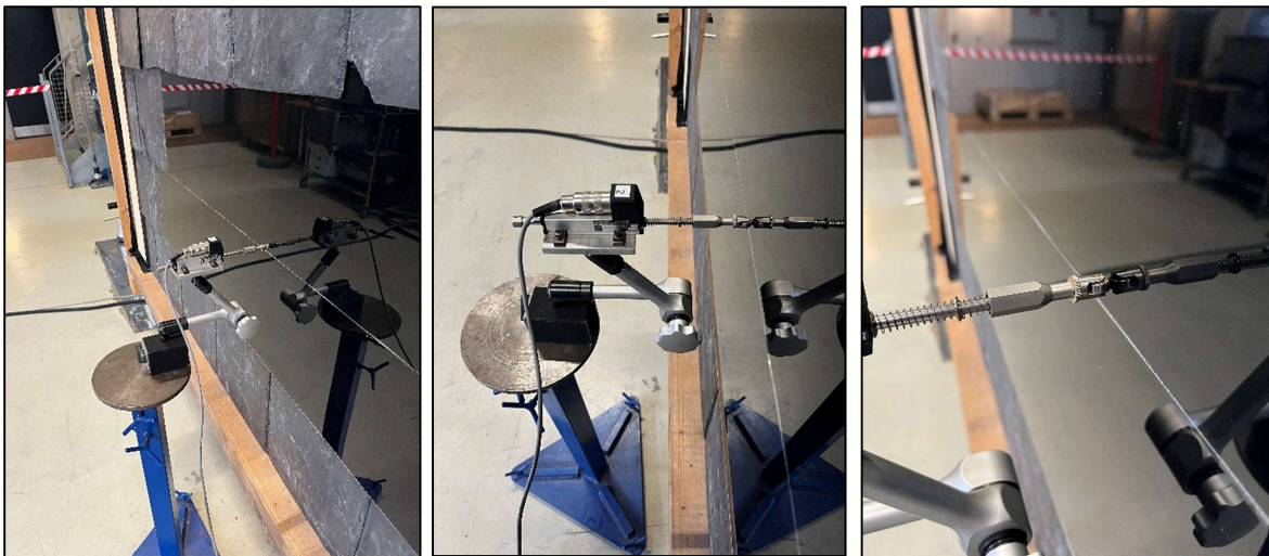
Figure 2 - The displacement sensor was mounted at the center of the test specimen.
