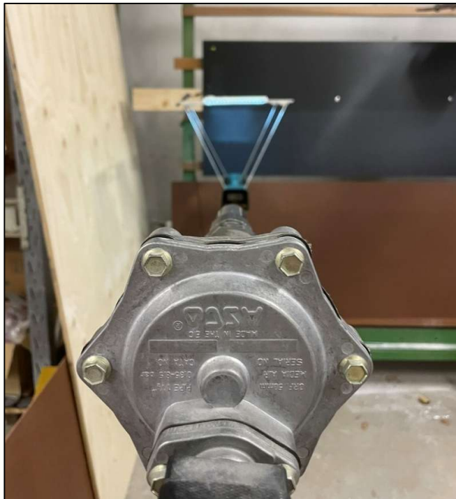
Figure 9 – Test apparatus and photoelectric velocity measuring system.
