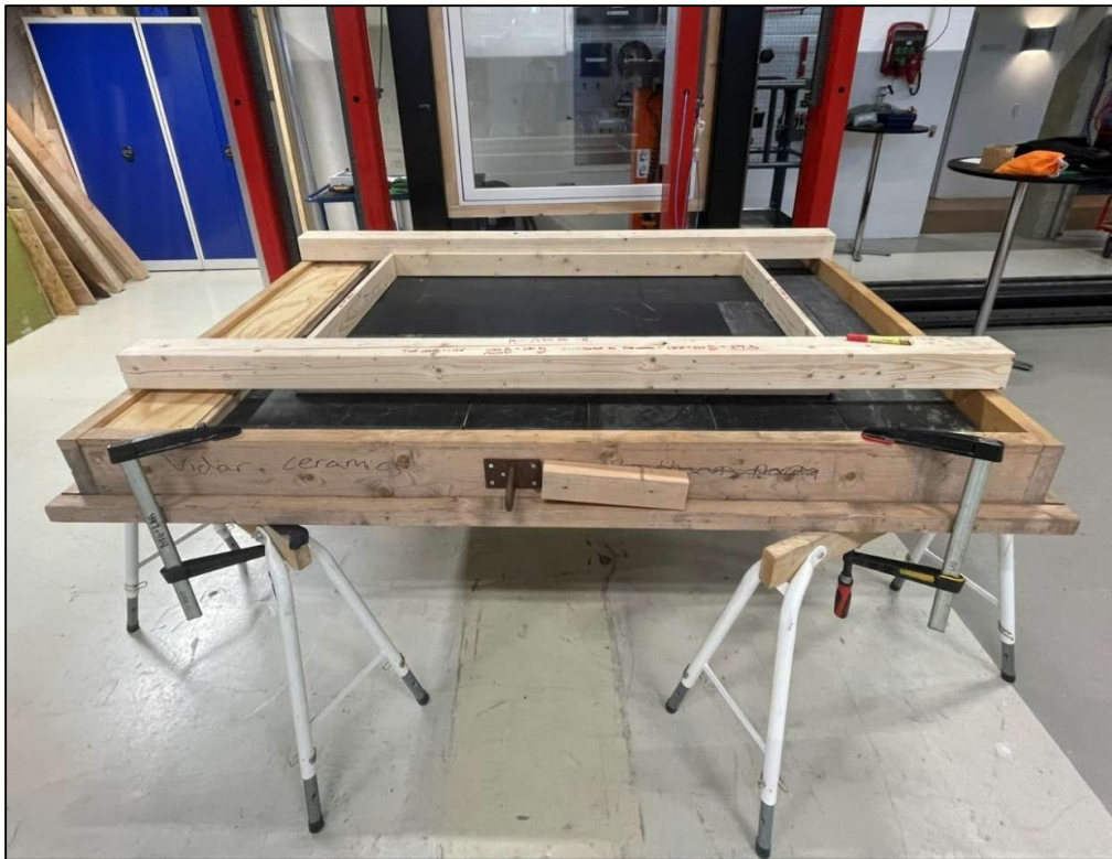
Figure 5 – Test setup for snow load.
