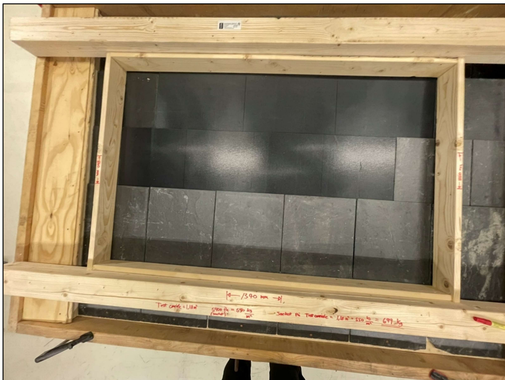
Figure 6 – Ekstra test frame to control the loading area.
